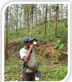
Figure 01, Measuring Tree Height by using Clinometers
